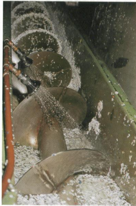
Archimedes' screw is still used today. Here an Archimedes' screw moves plastics through a modern recycling plant.
