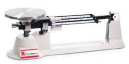
A <u>beam balance (triple)</u> is a tool used to measure the mass of an object.
