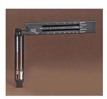
A <u>sling psychrometer</u> is a tool used to measure relative humidity by using two thermometers—a wet bulb and a dry bulb.
