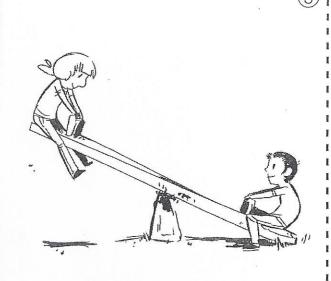
A lever is a bar that pivots or turns on a fixed point. The fixed point is called the fulcrum.
