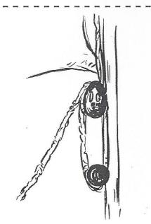
A pulley is a wheel that is used with a cord or rope. When you pull it downward, the other end lifts upward.
